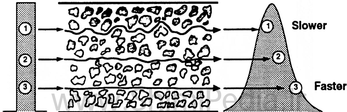
$$H = A + B/u + (C_{\text{lig}} + C_{\text{gas}})u$$
